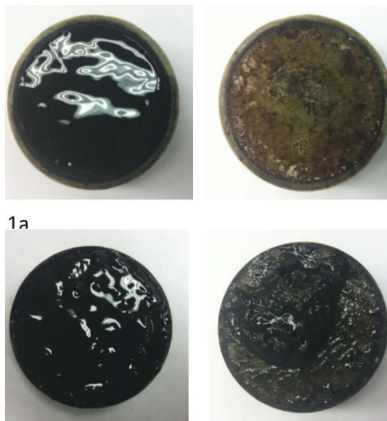
FIGURE 1. Filter cake (1a, top) is shown before (left) and after (right) MudOut treatment. The filter cake (1b, bottom) can be seen before (left) and after (right) formic acid treatment. (Source: EthicalChem)
